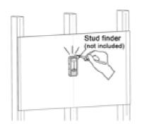
Step 1:Locate the timber stud behind the plaster and mark a vertical line at its center.
