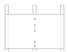
Step 3:Drill pilot holes at the marked locations using an 8mm drill bit.
