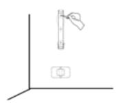
Step 1:Position the bike hanger and rear tyre guide at the recommended height and mark the hole positions.
