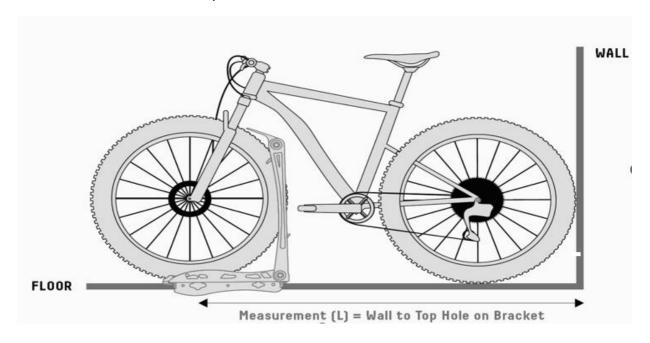
Step 2: Mark a point 75mm higher than dimension L from the ground. This will serve as the position for the top center hole.
