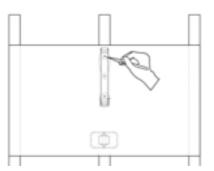
Step 2:Position the bike rack and rear tire guide at the recommended height, then mark the hole positions.
