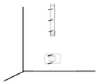
Step 4:Attach the bike hanger and rear tyre guide using the provided screws.
