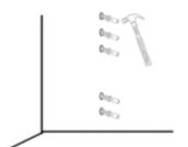
Step 3:Insert anchors into the holes and tap them in until flush with the wall.
