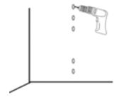
Step 2:Drill pilot holes at the marked locations using an 8mm drill bit.
